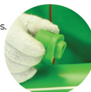
Protruding layers of saddle fitting after heating
